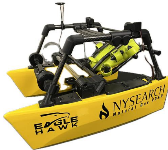
Figure 58: Aquatic Drones Perform Inspections of Submerged Pipelines
